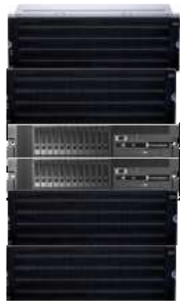
GSS 24: Light and Fast 2x3650 servers + 4xJBOD 20U rack 10 GB/Sec
