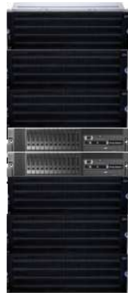
GSS 26: HPC Workhorse 2x3650 servers + 6xJBOD Enclosures, 28U 12 GB/sec
