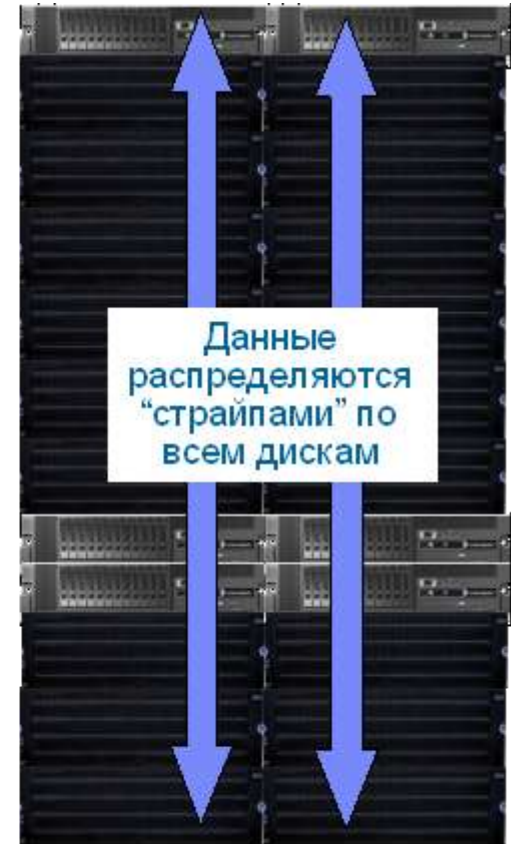
High-Density HPC Option 6x3650 servers + 18xJBOD 2x-42U Standard Racks 36 GB/sec
